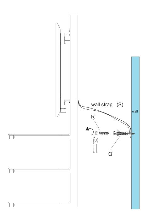
10- Place wall strap (S) at desired position on the wall. Mark the hole position with a pencil. Drill a hole on the pencil mark made on the wall with a 10mm size Drill Bit. Insert plastic anchor(Q) into the wall. Fasten the wall strap(S) to the wall by inserting screw(R) through grommet in nylon strap(S) and then into wall anchor.
